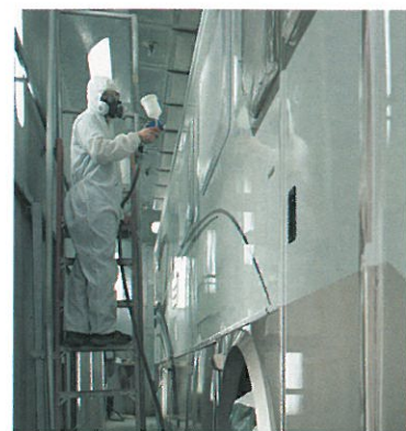
Above: Monaco continues to add value to your coach with a comprehensive paint procedure. Three layers of clear coat provide UV-ray protection and help insure the beauty of your coach with minimal maintenance for years to come.
