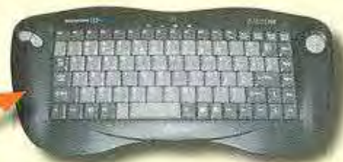
Wireless keyboard with radio frequency allows for use on all coach TV's. The on-board computer can be displayed on any of the four TVs and the non-line of sight wireless keyboard & mouse can be used up to 100 feet away from its receiver.
