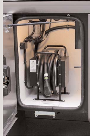
The optional 50-amp power cord reel provides easy storage of the power cord during and after use.
