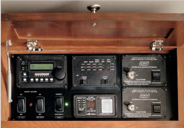
The specially designed Systems Control Center houses commonly used switches and controls in one convenient location at the front of the motorhome.
