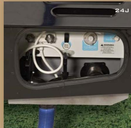
**EXTERIOR SERVICE CENTERS** The exterior service centers house water, drainage facilities and an available exterior wash station. Electrical center hookups also can be found here, including a power cord with the QuickPort® service connection hatch (not available on the 24J shown here). This allows you to close the compartment door even when connected to hookups at the campground. Everything is color-coded for your convenience.
