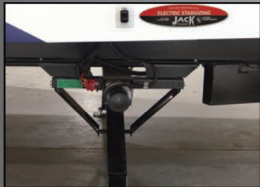
"One Touch" Electric Stabilizer Jacks reduce setup time
