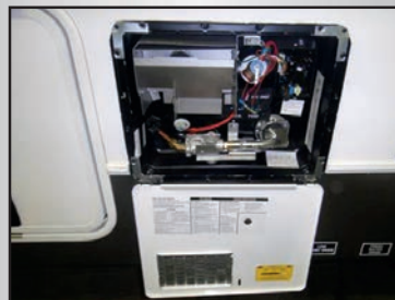
18 Gallon/Hour Quick Recovery Water Heater
