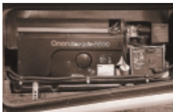
Flair's standard 4.0kW ultra-quiet Onan® generator provides 110V service and comes with a 3-year warranty. (Optional 5.5 kW generator shown.)
