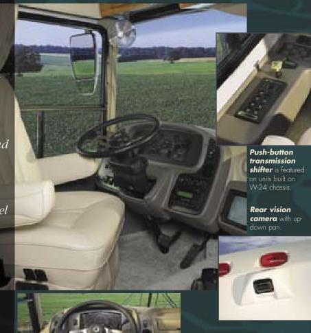
**Instruments** are clearly and intuitively labeled, and switches are illuminated for easy night time identification
