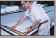
All coach body panels are vacuum laminated for unequaled strength and durability. This process uses advanced adhesives and vacuum to bond the various components into a single, inseparable unit
