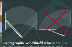
a wider swath of windshield than typical radial windshield wipers (right) of similar blade length.
