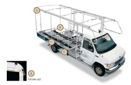
SUPERSTRUCTURE is the term given to Winnebago Industries' structural motor home design and construction. Rather than a single component, it is the culmination of design integration that incorporates steel and aluminum substructures; welded tubular steel floor risers; interlocking joint technology; and Thermo-Panel® floor, roof and sidewalls to form a high-strength, durable vehicle body.
