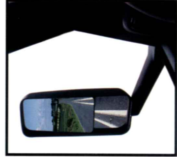
126-square inch-surface mirror including a 6x7 inch convex section on both mirrors.
