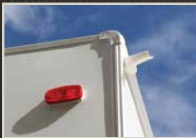
Drip rail with extra long drip spouts that help prevent black streaking.
