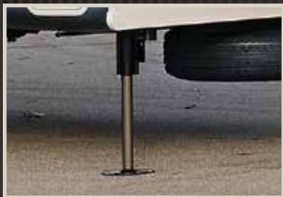
Wide stance power front jacks with quick release snap pins. (Optional hydraulic shown)
