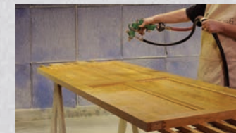
Clear-coated solid hardwood doors provide additional protection and luster
