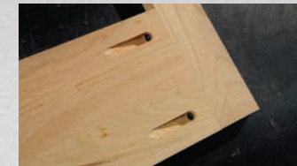
Pocket screws for structural integrity
