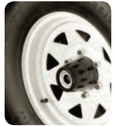
EZ lube axles provide a quick and easy way to grease your wheel bearings.
